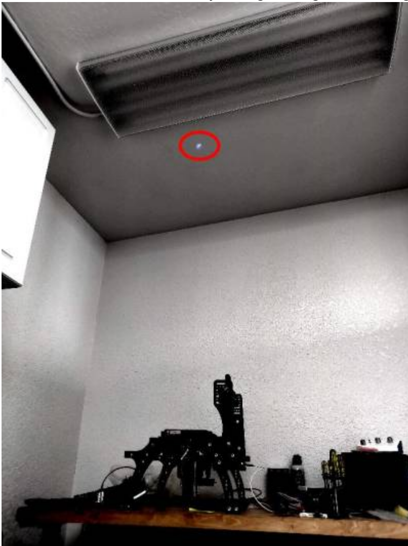
Collimated beam appears as a small bright dot on the ceiling
