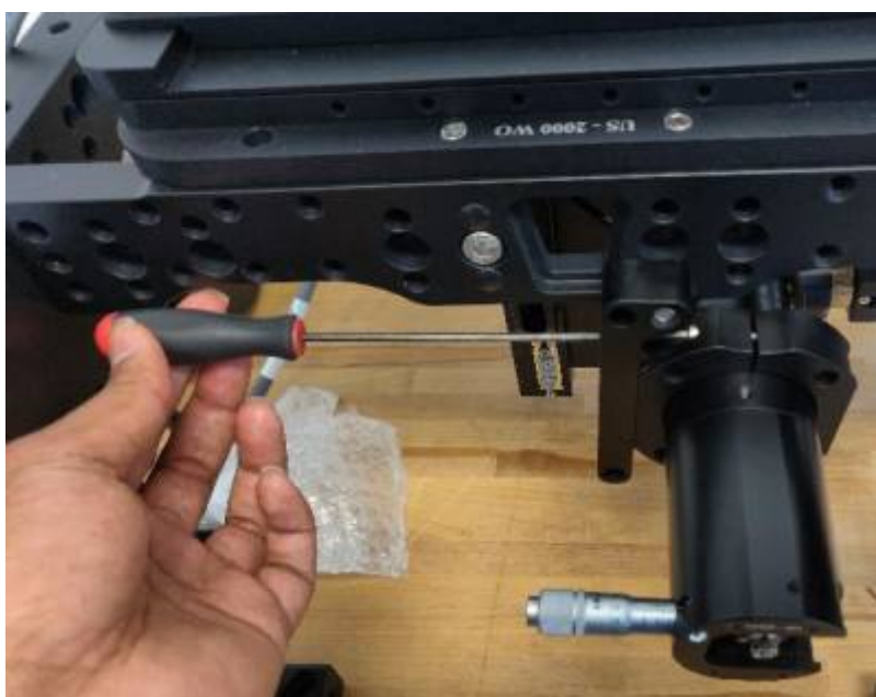
First screw to close the C support clamp
