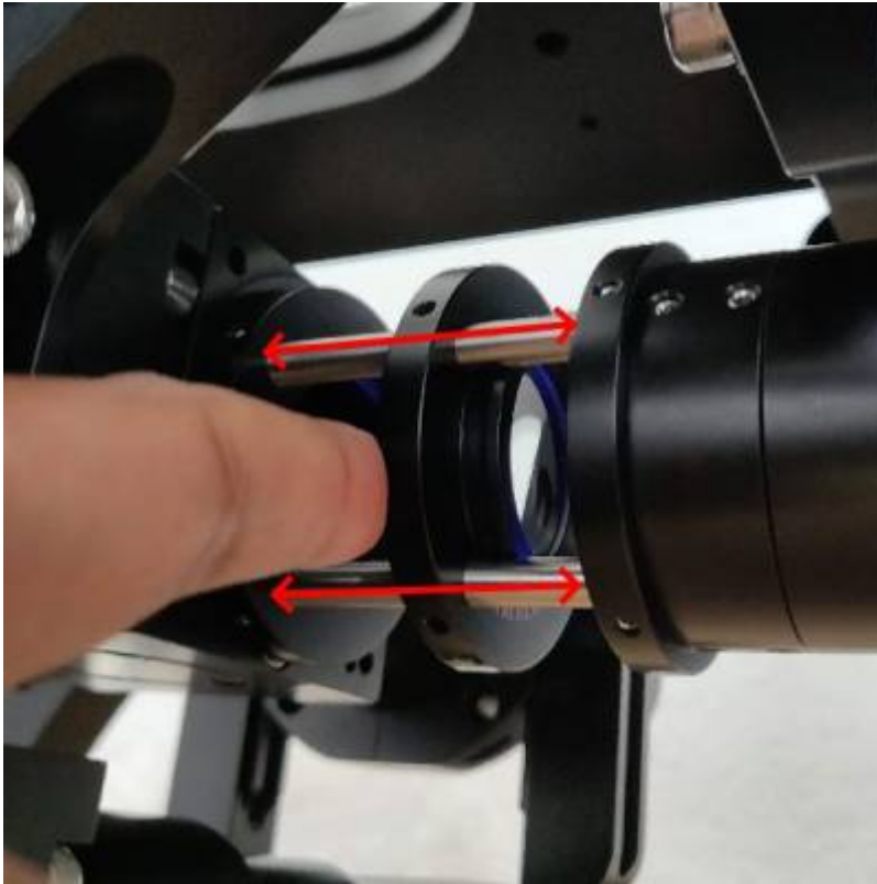
Focus the beam into the BFP by sliding the caged lens along the rails
