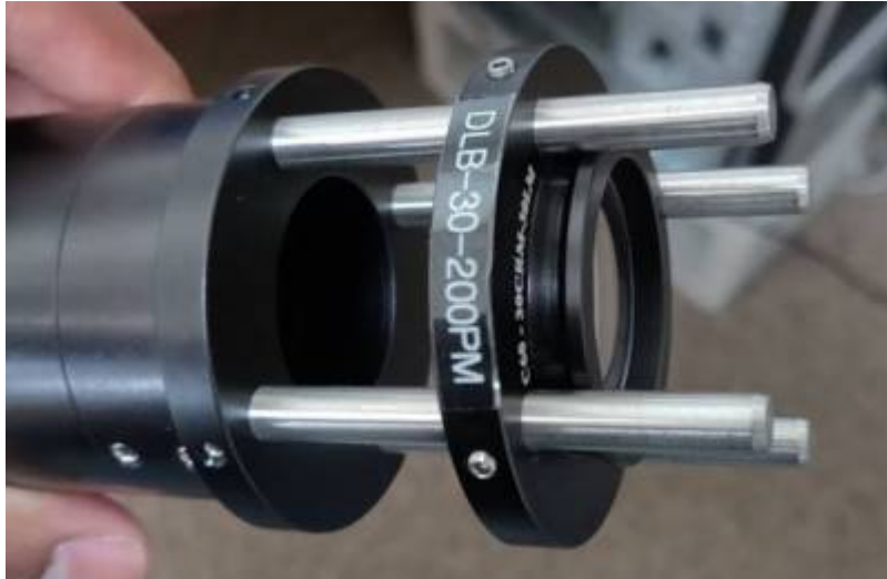
Install the focusing lens with the collar of the ring facing out / towards the RAMM
