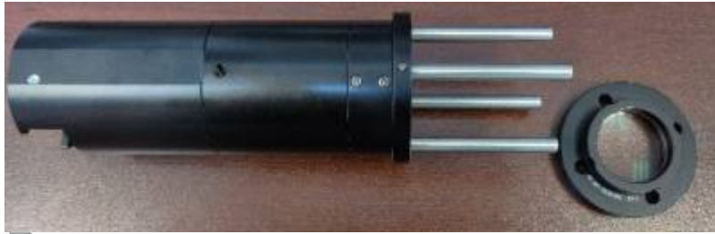
TIRF assembly with the ring-mounted focusing lens removed from the cage system
